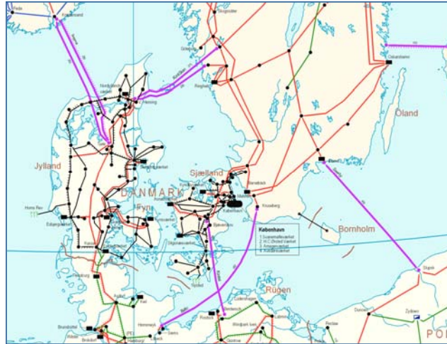
Fig. 36: Direct current submarine cables in the North and Baltic Sea (Source: UCTE, 2004)
