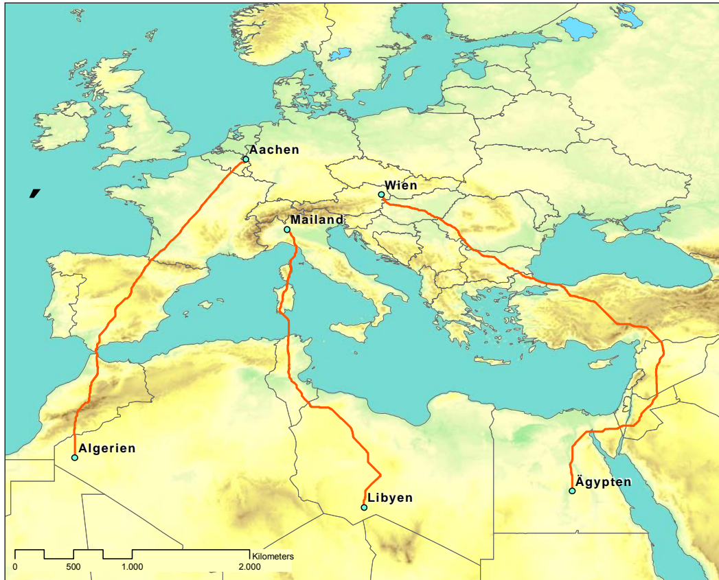
Fig. 55: Resulting course of HVDC lines for a solar electricity import.
